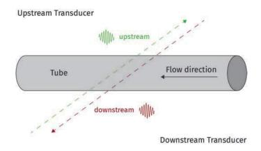
When sending ultrasonic sound signals through the measuring section, the transit time difference depends on the flow direction of the medium:
