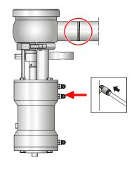
Weld it care/ try to make a stressless welding to avoid deformatin on sealing areas. Check the valve for regular operation after welding Only use pulsed arc welding and remember no gap between flange and tank plate.
