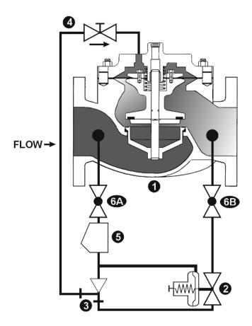
The Mark 5108 consists of the following components, arranged as shown on the schematic diagram:
