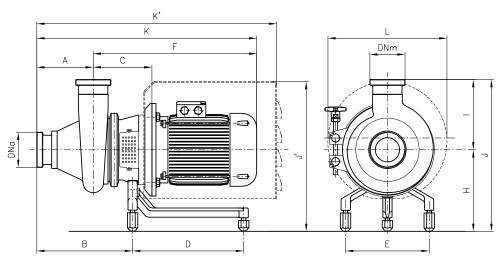
DN = DIN 11851 male threaded connection - Dimensions not binding - exec. with standard IEC/EN motors
