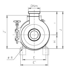
DN = DIN 11851 male threaded connection - Dimensions not binding - exec. with standard IEC/EN motors
